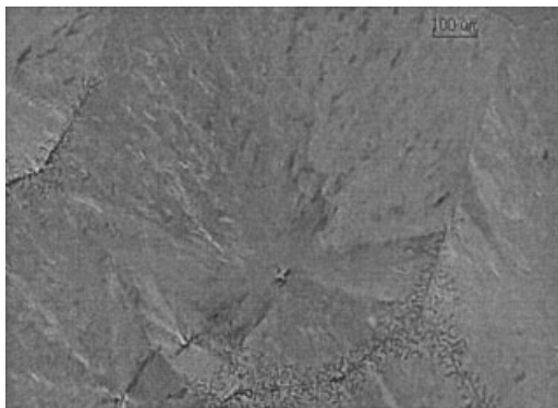
Figure 4 POM image of PEO spherulites under isothermal crystallization conditions with T_c = 45^\circ\text{C} .
